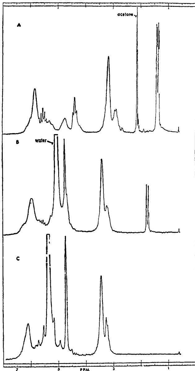
Figure 1. PMR spectra (a) in acetone- d_6 of [\text{Co}(\text{en})_2(\text{glyOCH}(\text{CH}_3)_2)](\text{ClO}_4)_3 ; (b) in \text{D}_2\text{O} of the 3+ adduct isolated following reaction of [\text{Co}(\text{en})_2(\text{glyOCH}(\text{CH}_3)_2)](\text{ClO}_4)_3 with glycine isopropyl esters in aqueous solution; (c) in \text{D}_2\text{O} of the 3+ adduct isolated following reaction of [\text{Co}(\text{en})_2(\text{glyOCH}(\text{CH}_3)_2)](\text{ClO}_4)_3 with aminoacetonitrile in aqueous solution (reference, TMS).
